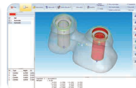
Automatic slicing of imported geometry
