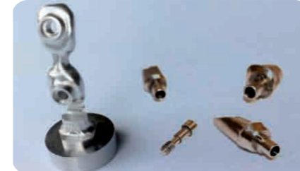
Automatic 5 Axis undercuts machining
