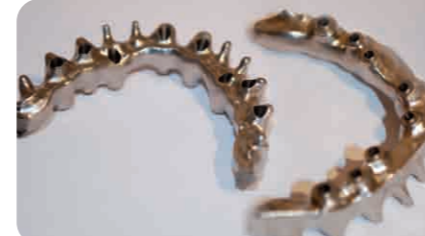
Titanium Implant bar machining on 5 Axis machine
